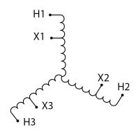
Three Phase Autotransformer with a capacity of 1500kVA, transforming 415Y Volts to 575Y Volts
