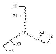
Three Phase Autotransformer with a capacity of 500kVA, transforming 575Y Volts to 200Y Volts
