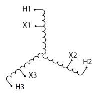
Three Phase Autotransformer with a capacity of 600kVA, transforming 400Y Volts to 240Y Volts
