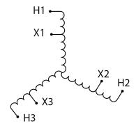
Three Phase Autotransformer with a capacity of 1000kVA, transforming 200Y Volts to 400Y Volts
