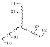
Three Phase Autotransformer with a capacity of 1000kVA, transforming 347Y Volts to 400Y Volts
