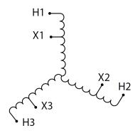
Three Phase Autotransformer with a capacity of 300kVA, transforming 600Y Volts to 120Y Volts
