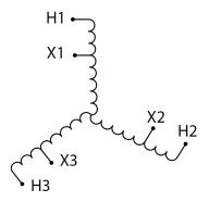
Three Phase Autotransformer with a capacity of 500kVA, transforming 415Y Volts to 200Y Volts
