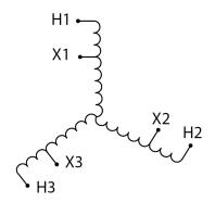
Three Phase Autotransformer with a capacity of 1500kVA, transforming 575Y Volts to 600Y Volts
