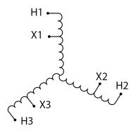
Three Phase Autotransformer with a capacity of 30kVA, transforming 415Y Volts to 120Y Volts
