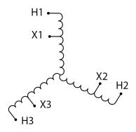
Three Phase Autotransformer with a capacity of 112.5kVA, transforming 600Y Volts to 480Y Volts
