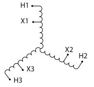
Three Phase Autotransformer with a capacity of 500kVA, transforming 277Y Volts to 220Y Volts
