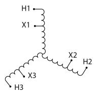
Three Phase Autotransformer with a capacity of 450kVA, transforming 110Y Volts to 200Y Volts
