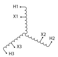
Three Phase Autotransformer with a capacity of 1000kVA, transforming 600Y Volts to 480Y Volts
