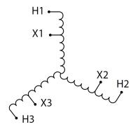
Three Phase Autotransformer with a capacity of 450kVA, transforming 208Y Volts to 220Y Volts
