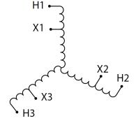
Three Phase Autotransformer with a capacity of 112.5kVA, transforming 600Y Volts to 550Y Volts
