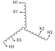
Three Phase Autotransformer with a capacity of 6kVA, transforming 115Y Volts to 347Y Volts
