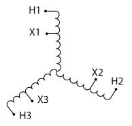
Three Phase Autotransformer with a capacity of 750kVA, transforming 240Y Volts to 416Y Volts
