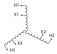
Three Phase Autotransformer with a capacity of 750kVA, transforming 460Y Volts to 416Y Volts
