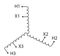
Three Phase Encapsulated Autotransformer with a capacity of 6kVA, transforming 480Y Volts to 208Y Volts
