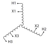
Three Phase Encapsulated Autotransformer with a capacity of 6kVA, transforming 480Y Volts to 208Y Volts
