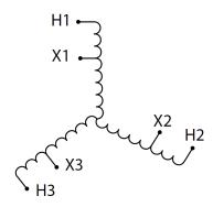
Three Phase Encapsulated Autotransformer with a capacity of 75kVA, transforming 600Y Volts to 480Y Volts
