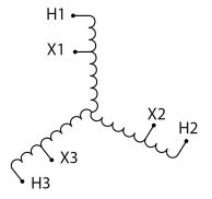
Three Phase Autotransformer with a capacity of 2500kVA, transforming 240Y Volts to 200Y Volts
