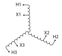
Three Phase Encapsulated Autotransformer with a capacity of 300kVA, transforming 600Y Volts to 480Y Volts
