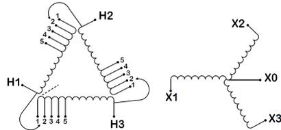
Three Phase Isolation Transformer with a capacity of 75kVA, transforming 600 Volts to 220Y/127 Volts
