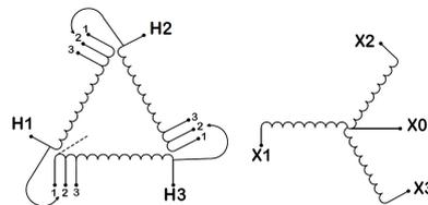
Three Phase Isolation Transformer with a capacity of 9kVA, transforming 347 Volts to 240Y/139 Volts
