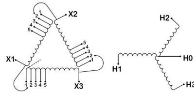
Three Phase Isolation Transformer with a capacity of 75kVA, transforming 550 Volts to 575Y/332 Volts
