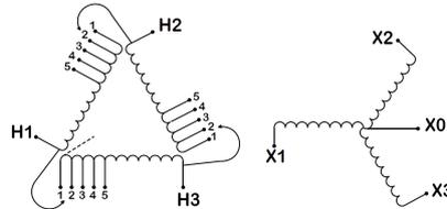
Three Phase Isolation Transformer with a capacity of 75kVA, transforming 550 Volts to 380Y/220 Volts
