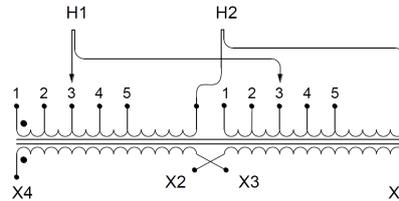
Single Phase Isolation Transformer with a capacity of 75kVA, transforming 480 Volts to 230/460 Volts
