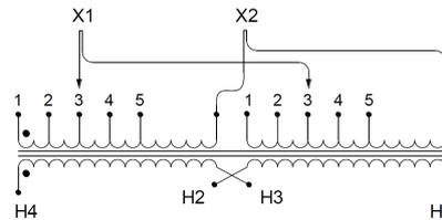
Single Phase Isolation Transformer with a capacity of 75kVA, transforming 416 Volts to 460 Volts
