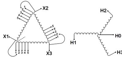
Three Phase Isolation Transformer with a capacity of 75kVA, transforming 347 Volts to 460Y/266 Volts
