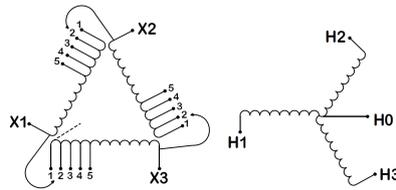
Three Phase Isolation Transformer with a capacity of 75kVA, transforming 208 Volts to 208Y/120 Volts
