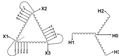
Three Phase Isolation Transformer with a capacity of 75kVA, transforming 120 Volts to 415Y/240 Volts
