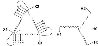
Three Phase Isolation Transformer with a capacity of 75kVA, transforming 120 Volts to 380Y/220 Volts
