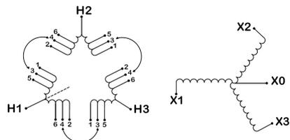
Three Phase Isolation Transformer with a capacity of 750kVA, transforming 600 Volts to 550Y/318 Volts
