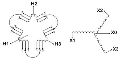
Three Phase Isolation Transformer with a capacity of 750kVA, transforming 600 Volts to 416Y/240 Volts
