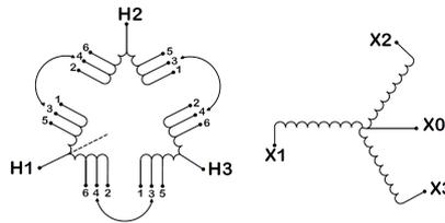
Three Phase Isolation Transformer with a capacity of 750kVA, transforming 600 Volts to 380Y/220 Volts
