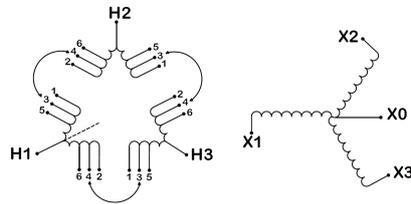
Three Phase Isolation Transformer with a capacity of 750kVA, transforming 600 Volts to 230Y/133 Volts
