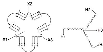
Three Phase Isolation Transformer with a capacity of 750kVA, transforming 440 Volts to 550Y/318 Volts
