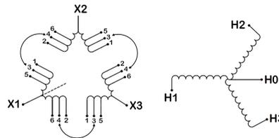
Three Phase Isolation Transformer with a capacity of 750kVA, transforming 380 Volts to 480Y/277 Volts
