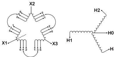
Three Phase Isolation Transformer with a capacity of 750kVA, transforming 208 Volts to 220Y/127 Volts
