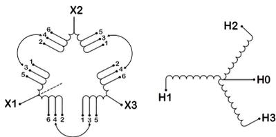
Three Phase Isolation Transformer with a capacity of 750kVA, transforming 208 Volts to 208Y/120 Volts
