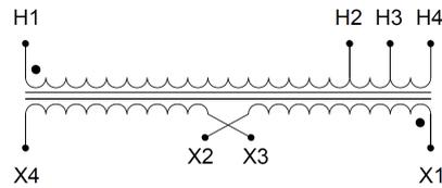
Single Phase Isolation Transformer with a capacity of 7.5kVA, transforming 575 Volts to 120/240 Volts
