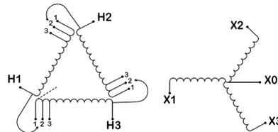
Three Phase Isolation Transformer with a capacity of 6kVA, transforming 575 Volts to 550Y/318 Volts
