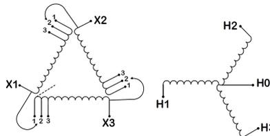
Three Phase Isolation Transformer with a capacity of 6kVA, transforming 220 Volts to 440Y/254 Volts
