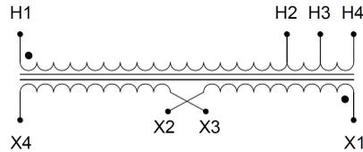
Single Phase Isolation Transformer with a capacity of 5kVA, transforming 480 Volts to 120/240 Volts
