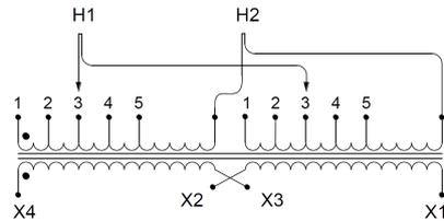
Single Phase Isolation Transformer with a capacity of 50kVA, transforming 550 Volts to 240/480 Volts
