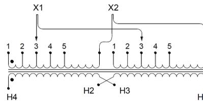
Single Phase Isolation Transformer with a capacity of 50kVA, transforming 415 Volts to 480 Volts
