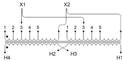
Single Phase Isolation Transformer with a capacity of 50kVA, transforming 277 Volts to 416 Volts
