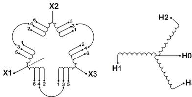
Three Phase Isolation Transformer with a capacity of 500kVA, transforming 208 Volts to 550Y/318 Volts
