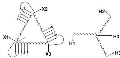
Three Phase Isolation Transformer with a capacity of 45kVA, transforming 400 Volts to 416Y/240 Volts
